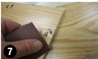
**7-** On the newly cut side of the board, sand (grit 120) at an angle of 45° to create a new "V" at the end of the board.
